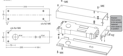
HINGE JAMB For front bracket, you have two options (1) or (2), depending on the fixing hole used. **(1**)
