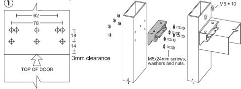
Select fixing holes most suitable for section and drill clearance size for M5 screws.
