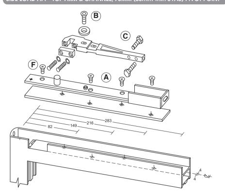
Prepare the top rail of the door as detailed, ensuring that the internal faces of the stile and top rail have been cut away to enable the closer spindle to be engaged during door
