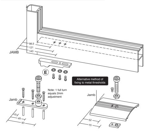
Prepare the bottom rail of the door to accommodate the pivot shoe with 2 No. drilled and tapped M6 holes at 98.5mm and 143mm centres. Fit pivot shoe to underside of door, through the slotted holes with 2 No. M6 x 16mm round head screws and lock-washers **(E)**.
