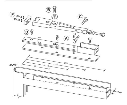
Prepare the top rail of the door as detailed, ensuring that the internal faces of the stile and top rail have been cut away to enable the closer spindle to be engaged during door
