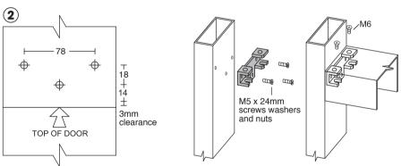
Select fixing holes most suitable for section and drill clearance size for M5 screws.
